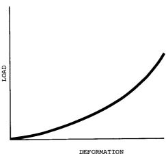
FIG. 3 Procedure B—Increasing Stiffness
