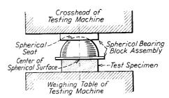
FIG. 4 Spherical Bearing Block for Compressive Strength Test
