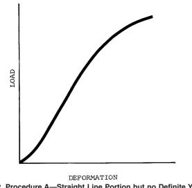
FIG. 2 Procedure A—Straight Line Portion but no Definite Yield Point
