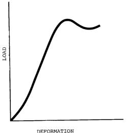
FIG. 1 Procedure A—Straight Line Portion with Definite Yield Point
